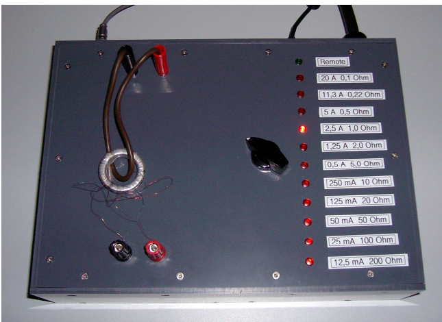
Ring measurement with remote switchable shunts IEC 60404-6
