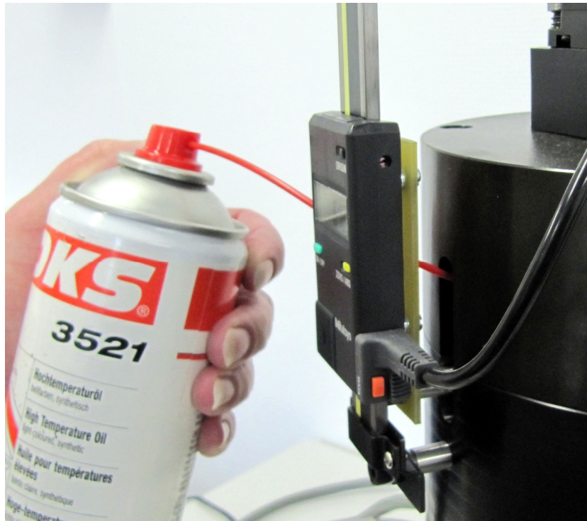
Oiling of upper cylinder
