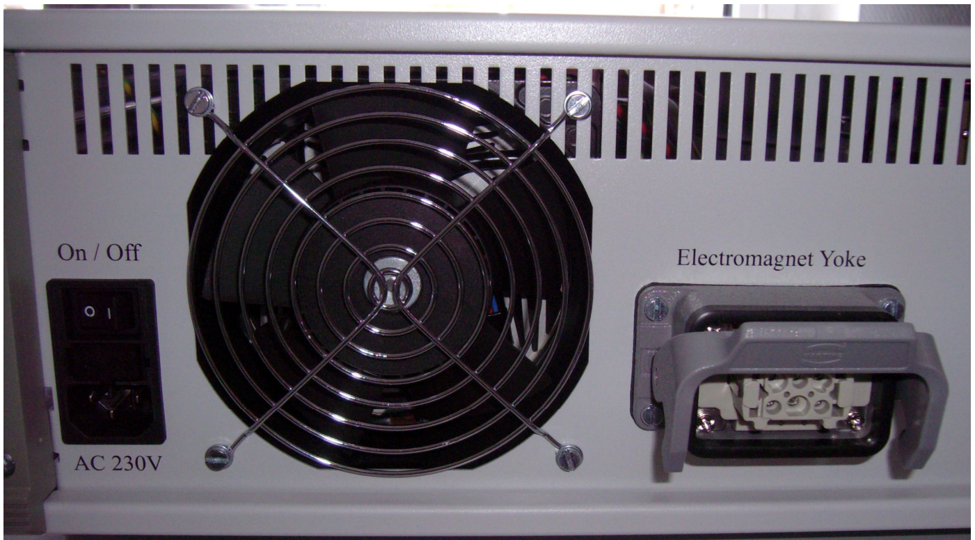
Line voltage input, power switch and the electromagnet yoke connector
