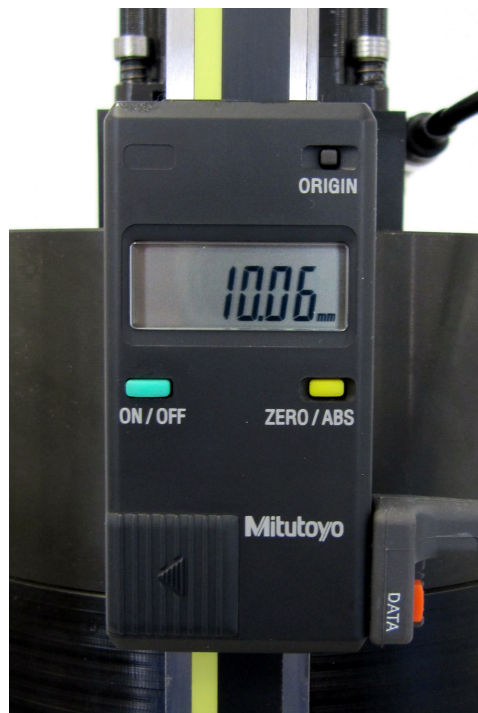
Digital caliper showing magnet thickness
