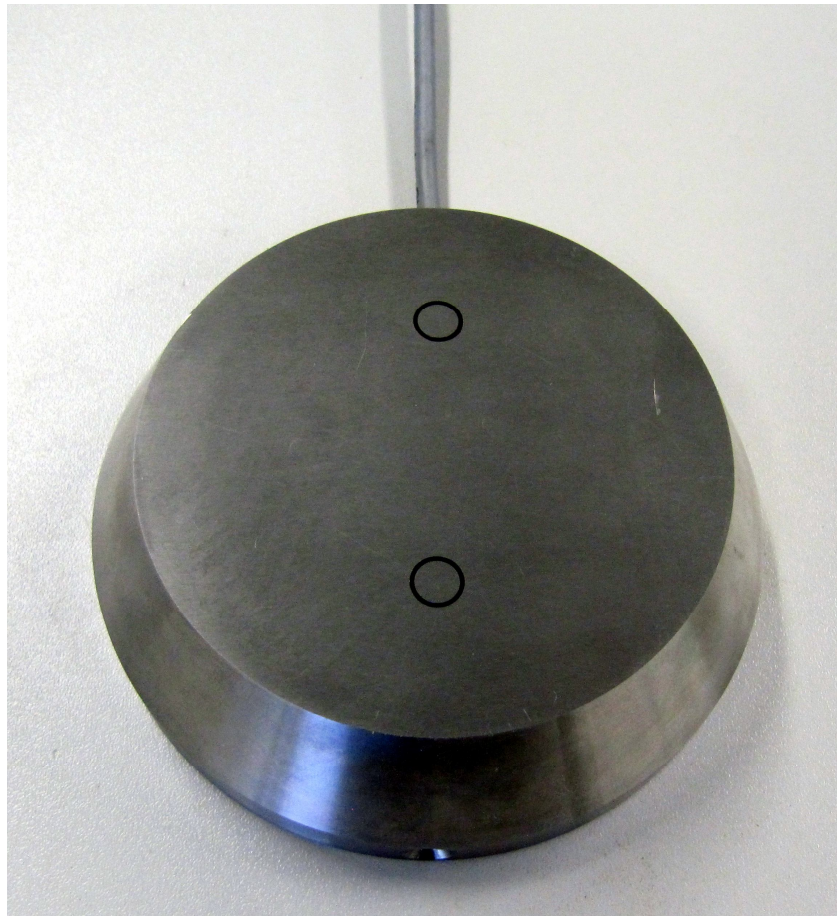
Flat pole shoes with embedded coils
